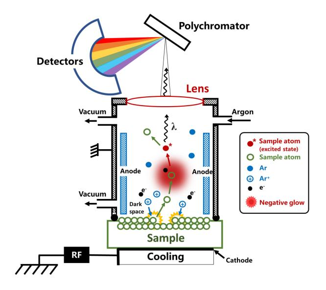
Schematic of a GD-OES instrument working principle
