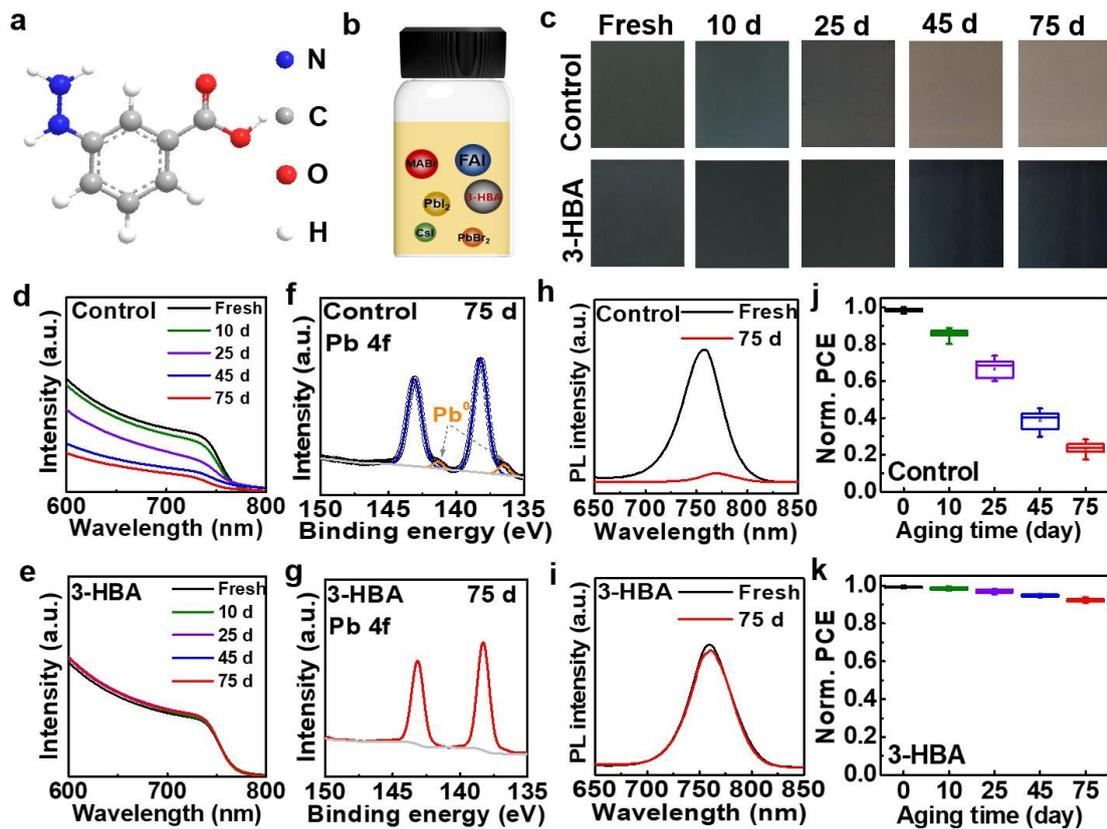
**Figure 1. Enhancing precursor stability and device reproducibility.** (a) Chemical structure of 3-HBA. (b) Schematic illustration of perovskite precursor solution incorporating 3-HBA. (c) Photographs of the perovskite films prepared by precursor
