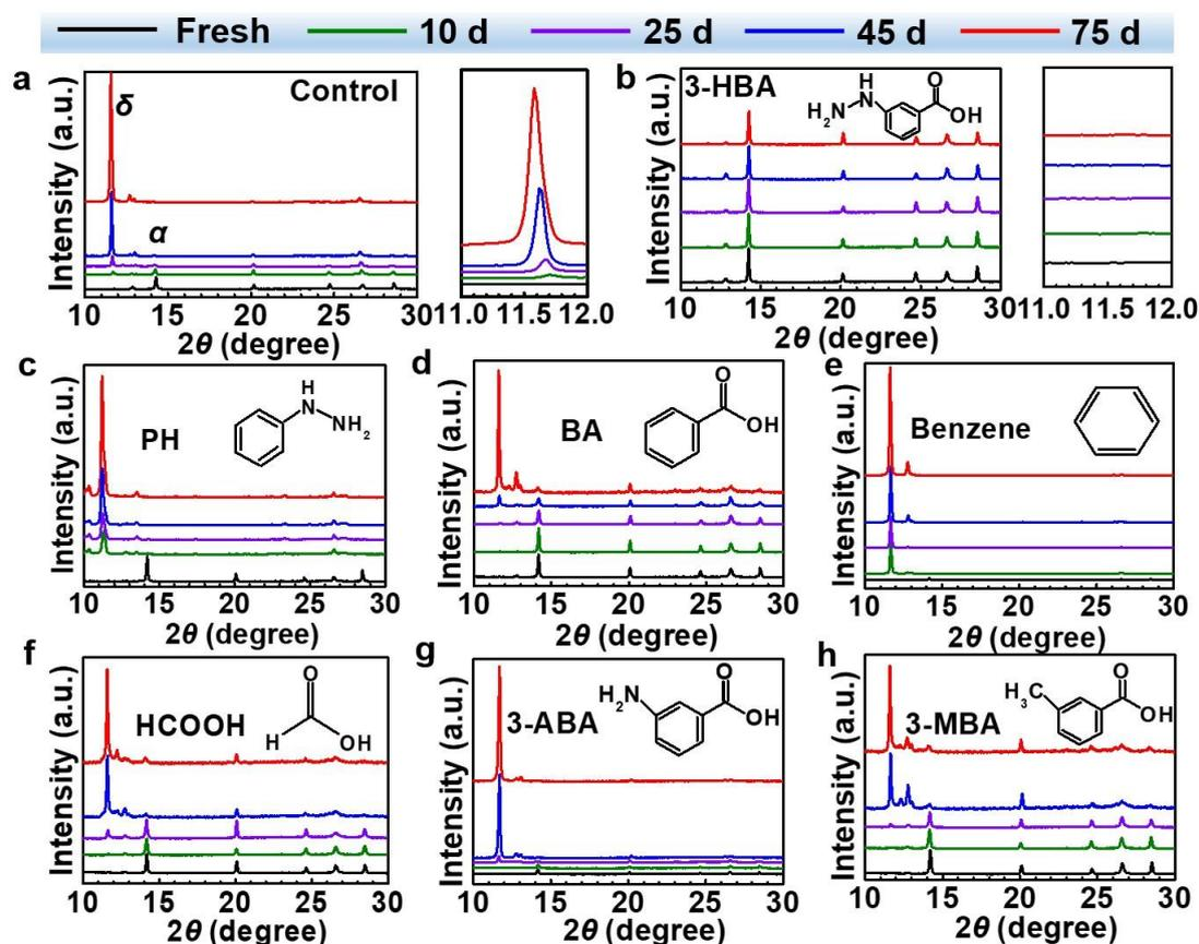
**Figure 2. Investigation of the effect of different functional groups on the phase stability of perovskite films.** (a) control, (b) with 3-HBA, (c) with PH, (d) with BA, (e) with C<sub>6</sub>H<sub>6</sub>, (f) with HCOOH, (g) with 3-ABA, and 3-MBA aged for different times. The illustration shows the chemical structures of the additive molecules.
